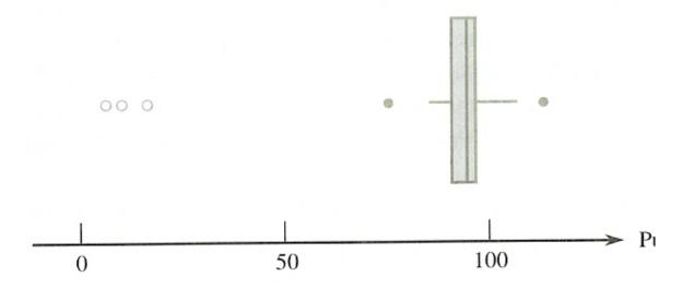
Figure 1.10: A box plot of the pulse width data showing mild (filled circles) and extreme outliers (blank circles).
