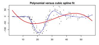
motorcycle data: time vs. head acceleration (red: cubic polynomial; blue: cubic splines)
